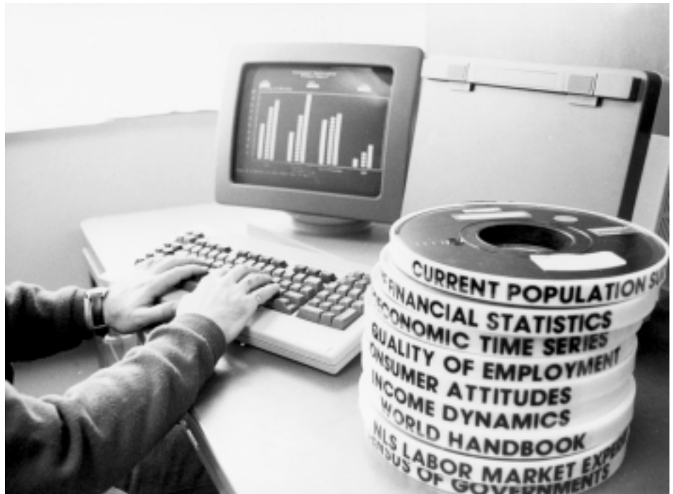
Working with magnetic data storage tapes.
